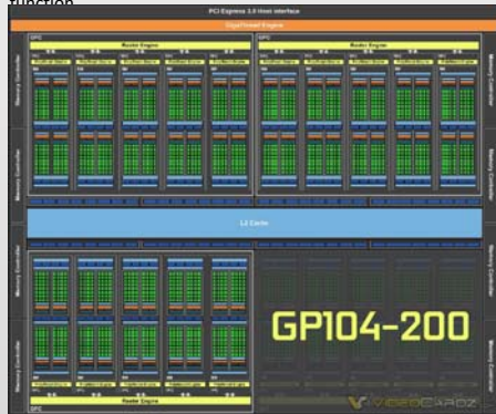
Diagram of the GP104 chip used in the GTX 1070 for testing. This chip features 1920 CUDA cores split between 15 SMs. There are 8 GB of VRAM associated with this card. For the experiment, 2 GTX 1080 Ti cards will be used.
